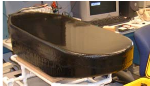
Figure 3: AUV Hull Fabrication
